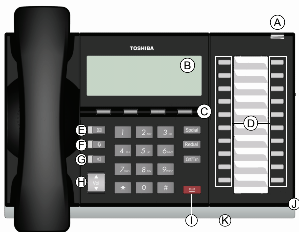
20 Programmable Feature Buttons 4-Line LCD
