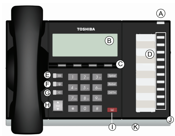
10 Programmable Feature Buttons 4-Line LCD
